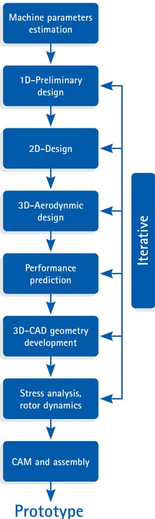
For the aerodynamic design, we use our competency in applying commercial flow solvers ANSYS, Numeca, and STARCCM+, as well as the research flow solver TRACE by the German Aerospace Center (DLR, Deutsches Zentrum für Luft- und Raumfahrt).
