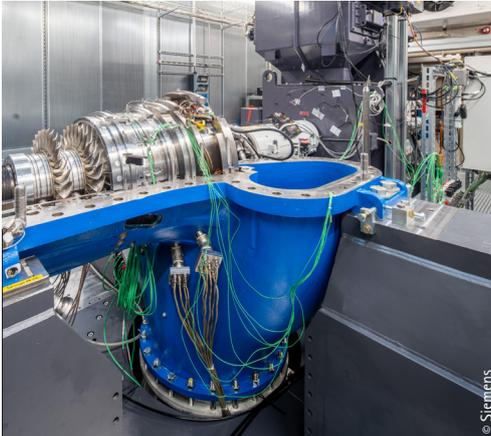
Multi-stage air turbine in preparation for aerodynamic experiments
