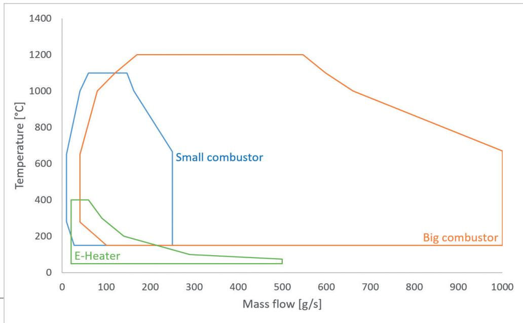
Operating ranges of the turbocharger test-facility for three heat sources
