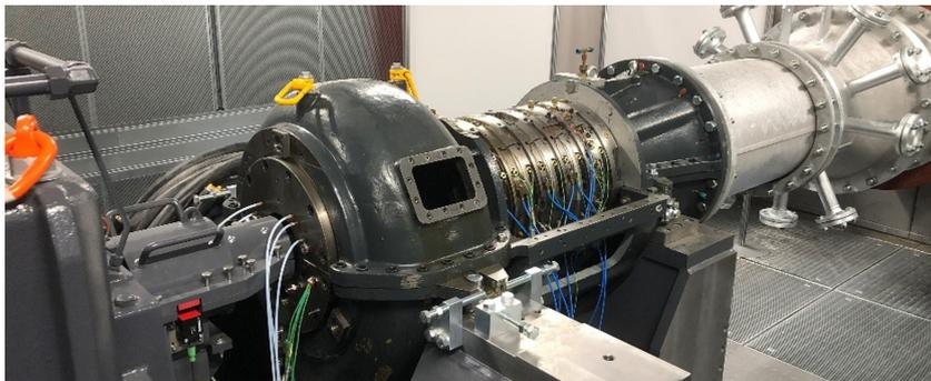
Four-stage high speed axial compressor
