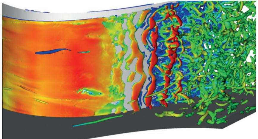
Vortex detection with Lambda-2 criterion of T161 profile by DNS
