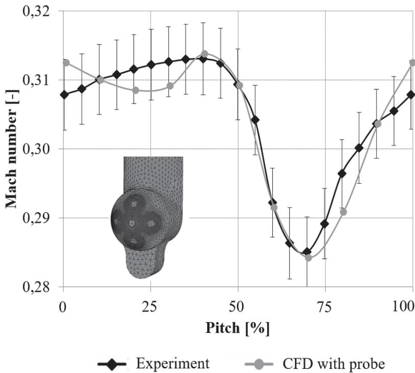
Post-Test CFD including the probe vs. experiment in a five-stage turbine (errorbars = 95% confidence interval)
