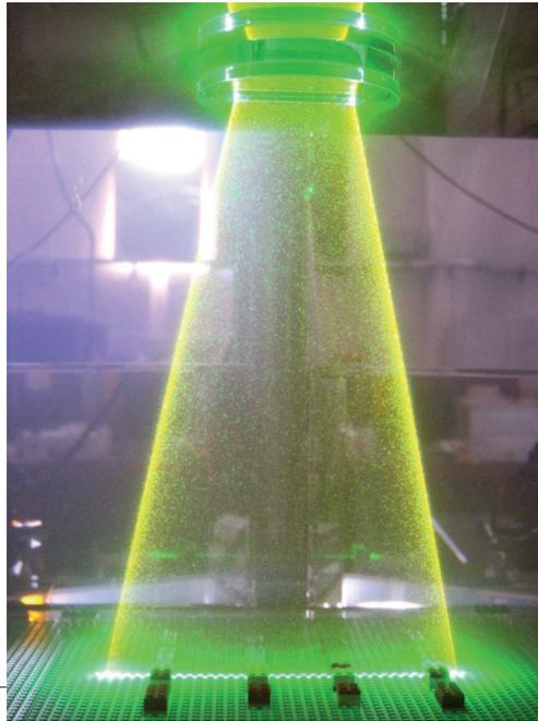
PIV light sheet in the water tunnel
