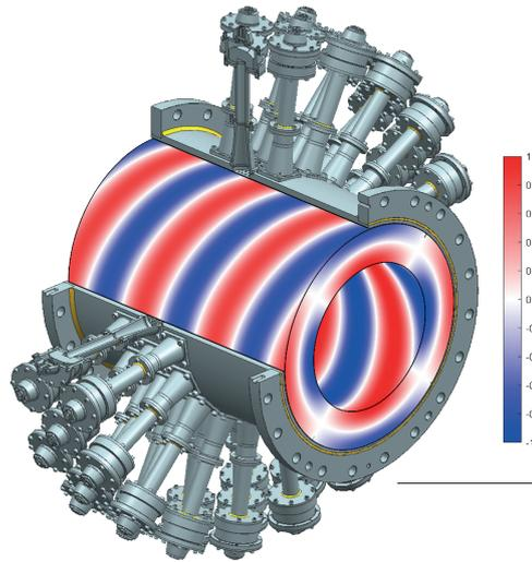
Schematic of three-row AWT's acoustic sound generators
