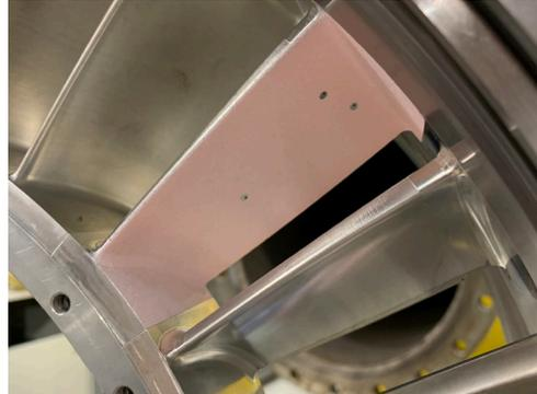
PSP-coated vane for measurements at the AWT
