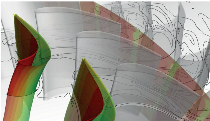
Analysis of rotor-stator interactions by unsteady flow simulations
