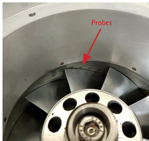
Probes in a rotor casing
