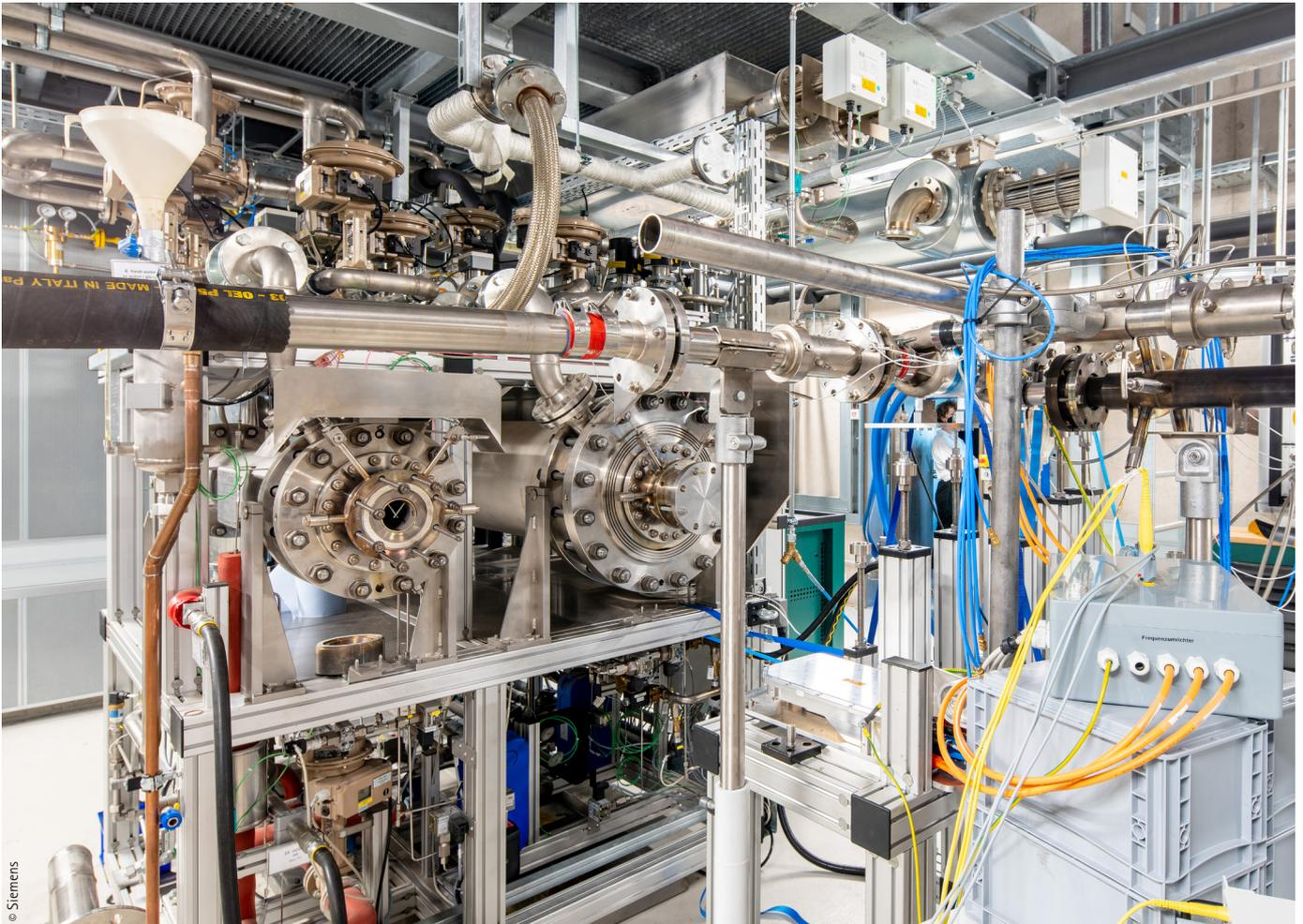
For research on exhaust gas turbochargers, turbocharging systems for fuel cells, and electrically driven compressor systems, we operate a test rig for turbocharging systems and electric air compressors. Our projects include the development of new turbocharging and compressor systems and the optimisation for existing applications. For the suc-
