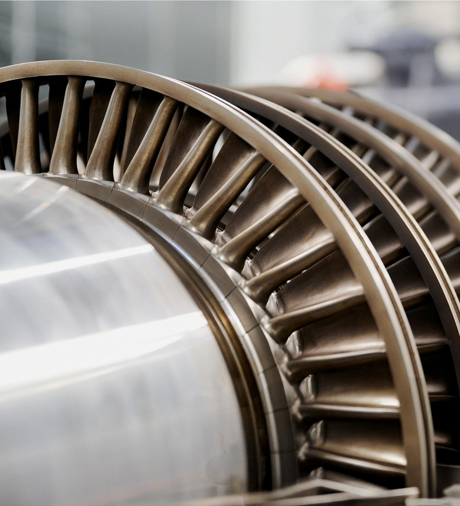
Four-stage high speed axial turbine
