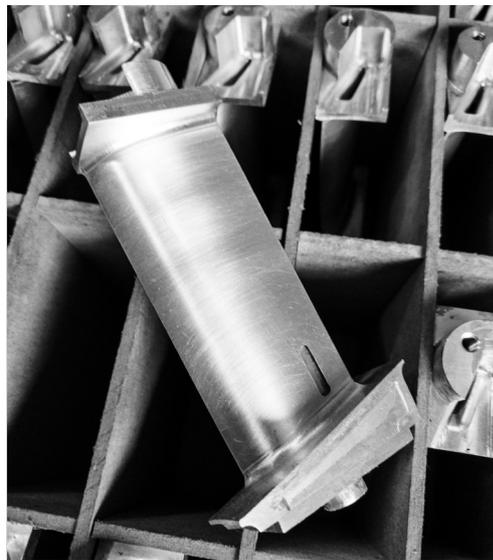
Stator vanes for active flow control
