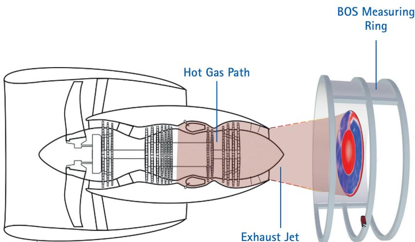
Schematic of the density measurement in the exhaust jet of a jet engine (red = low density, blue = high density)
