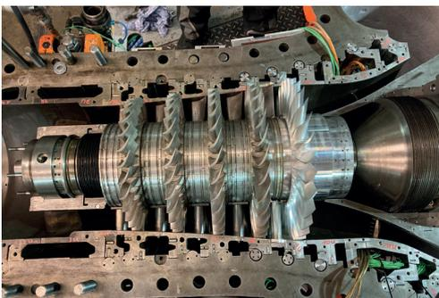
Five-stage gas turbine design for experiments in aeroelasticity
