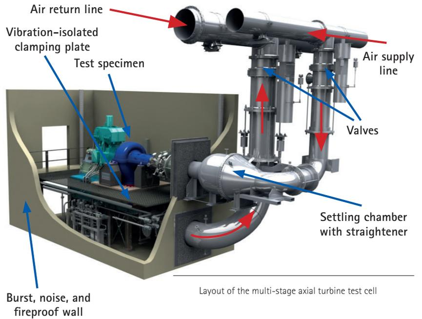
Layout of the multi-stage axial turbine test cell
