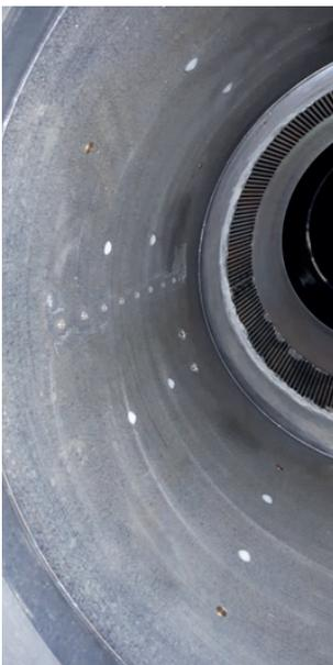
Microphone arrays placed in the shroud of the AWT
