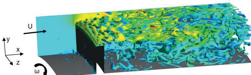
LES of the turbulent flow in a generic labyrinth seal
