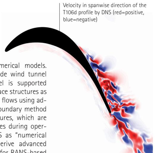
Velocity in spanwise direction of the T106d profile by DNS (red=positive, blue=negative)
