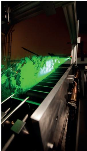
Linear Cascade Wind Tunnel with PIV light sheet
